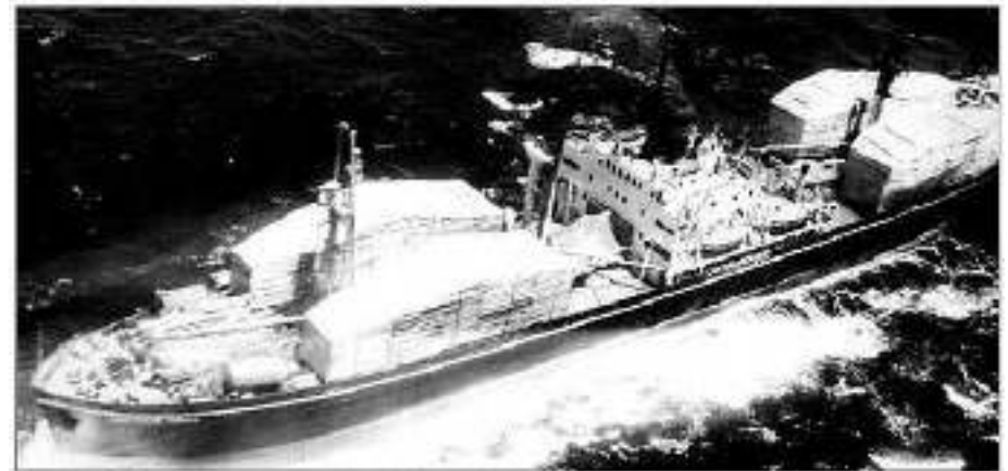
Figure 1. Soviet cargo ship carrying crated guided missile patrol boats.
